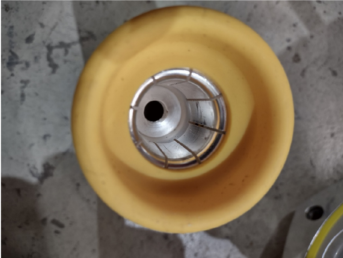
Picture 5 Contacts after short circuit test
