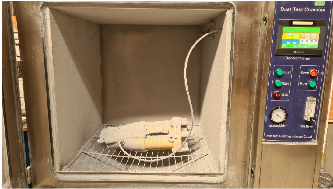
Picture 3 Coupler in dust test
