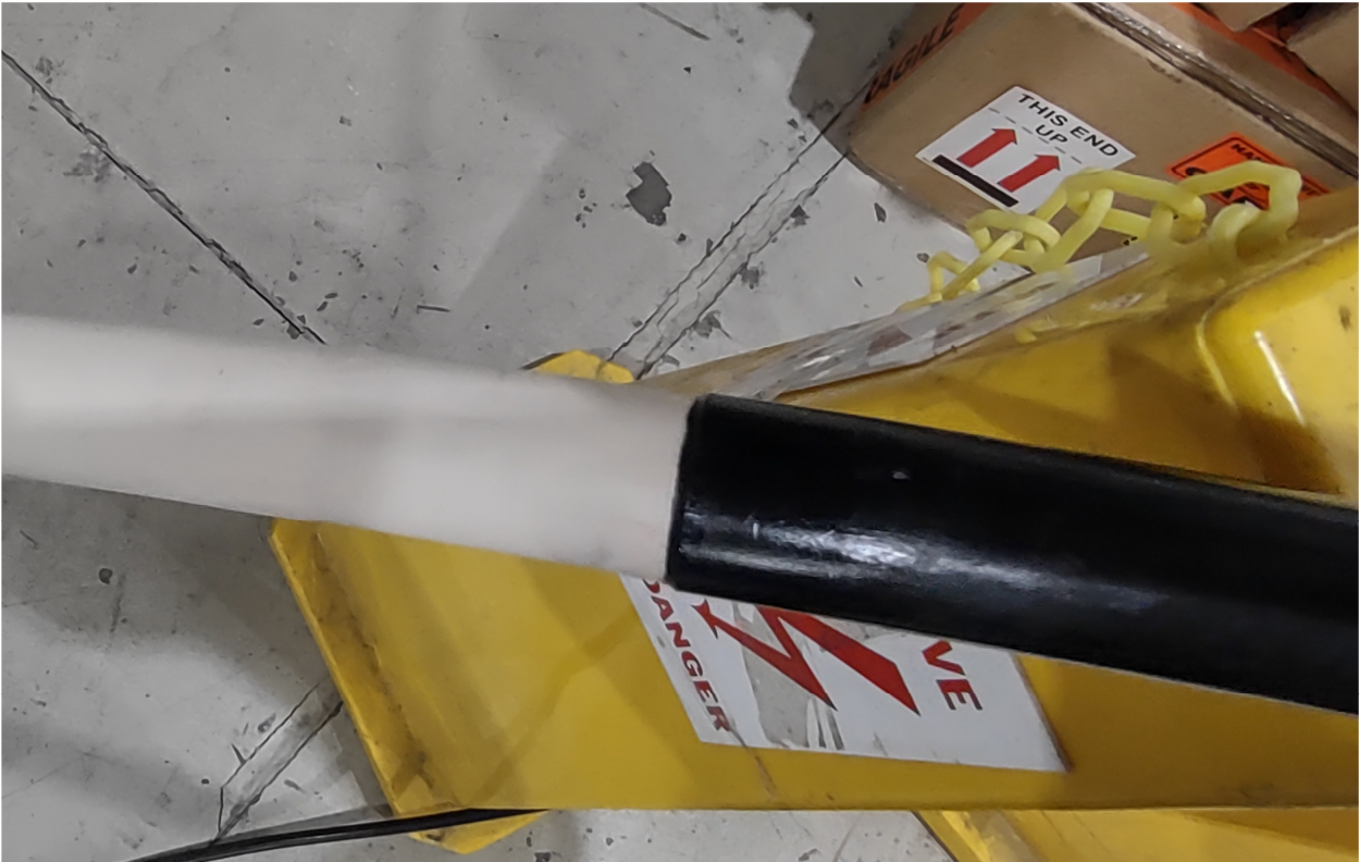
Picture 1 Cable sample, Cold Shrink Stress Relief Tube not installed
