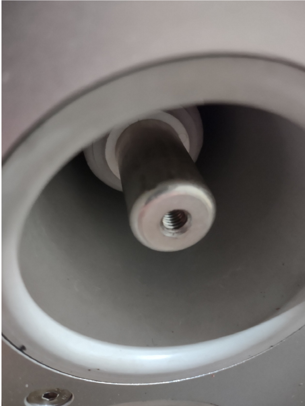
Picture 5 Contacts after short circuit test
