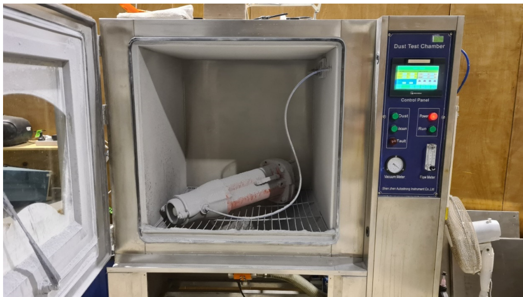
Picture 2 Coupler in dust test
